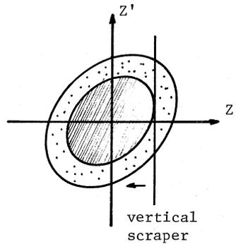
Fig. 2. A situation of the scraped beam in the vertical phase space diagram.
