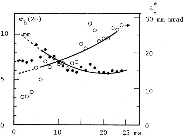
Fig. 4. Vertical beam size and vertical beam emittance vs. time during acceleration. Dotted line shows estimated curve. Beam blow up is appeared at 17 ms. Emittance grows continuously during acceleration.
