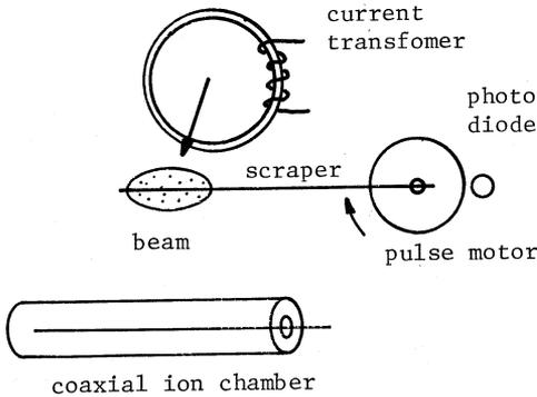
Fig. 1. A schematic diagram of the measurement for the vertical beam size in the booster synchrotron.
