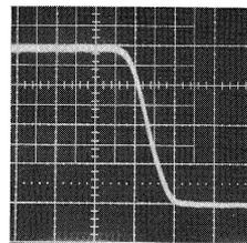
Fig. 3. A beam intensity variation at transit of the vertical scraper.
