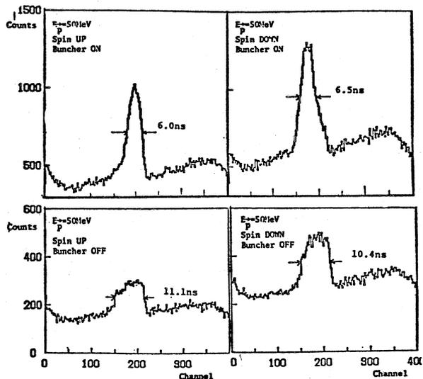
Fig. 2. Time structure of polarized proton
