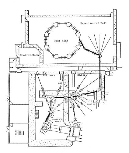
Fig. 1 The layout of the TEST RING and the beam transport system
