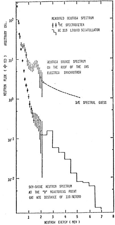
Fig. 4. ES Skyshine Neutron Spectrum
