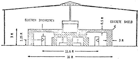
Fig. 1. Cross Sectional View of
