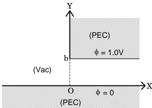
Figure 10: Geometry for the benchmark test. The hatched and white areas indicate PEC and vacuum regions, respectively. There is an infinitely sharp edge at  $(X, Y) = (0, b)$ . The minimum distance and potential difference between the two PEC regions are set to be  $b = 1.0$  mm and 1.0 V, respectively.
