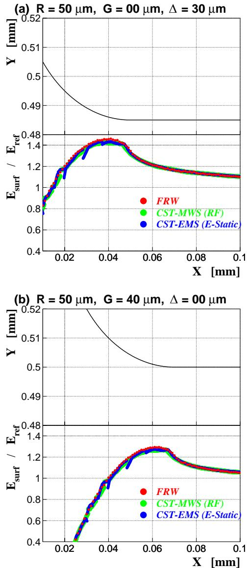
Figure 8: Conductor surfaces (top figures) and the surface electric-field strengths as a function of  $X$  (bottom figures). Each red point indicates a computation result using the FRW method.
