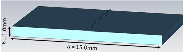
Figure 2: Vacuum region of the rectangular waveguide with a small groove at the center of the E-plane. The background material is PEC.
