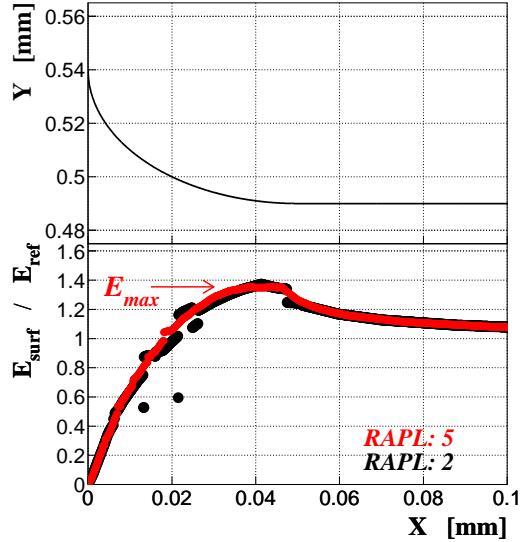
(b) Conductor surface (top) and the surface electric-field strength as a function of  $X$  computed with a RAPL value of 2 (black) or 5 (red) (bottom).
