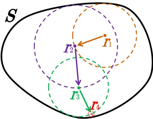
Figure 7: Schematic diagram of FRW. If  $r_4 < r_{\min}$ , this random walk is terminated, and the potential value at the nearest boundary is used.  $S$  indicates a boundary with known potentials.
