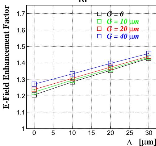
(a) For RF fields computed by using MWS.
