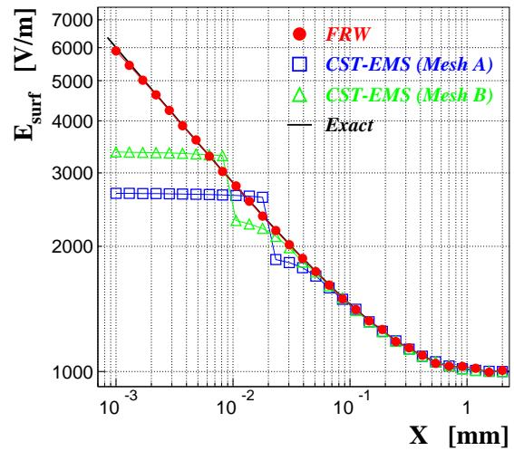
Figure 11: Surface electric-field strengths at  $Y = b$  as a function of  $X$  for the benchmark geometry shown in Fig. 10. Near the infinitely sharp edge located at  $(X, Y) = (0, b)$ , the mesh sizes in the Mesh A and B of the EMS computations are 36  $\mu$ m and 18  $\mu$ m, respectively. The solid line indicates an exact solution from the analytical formulae of Eq. (6) and (7).
