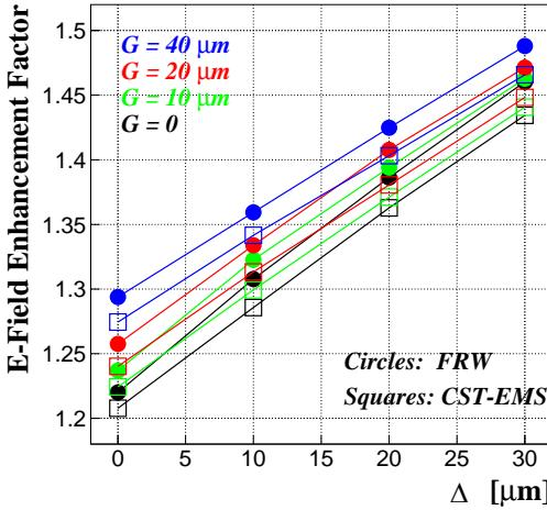
Figure 9: Electric-field enhancement factors as functions of  $G$  and  $\Delta$ . The circles (squares) indicate computation results by using the FRW method (EMS).
