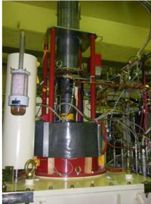
Fig.3 X-band (11.424 GHz) 50 MW Klystron
