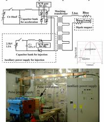
Figure 4: Auxiliary power supply has been connected to the pulse power supply in parallel at the primary winding of the matching transformer.
