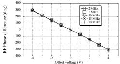
Figure 8: Preliminary phase feedback test on its linearity.
