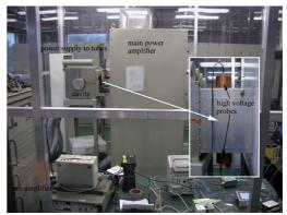
Figure 9: Developed RF high power system. Compact cavity is connected to the power amplifier in the middle. Pre-amplifier is at the left bottom corner and DC power supply to the main amplifier is in the rear.
