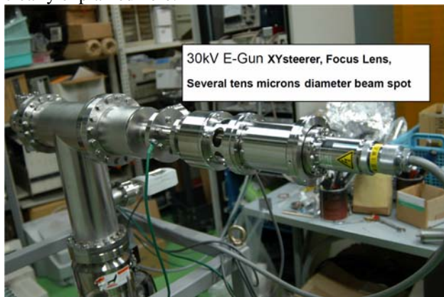
Figure 4: 30kV E-Gun XYsteerer, focus lens, several tens microns diameter beam spot.
