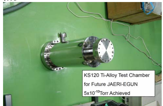
Figure 6: KS120 Ti-alloy test chamber for future JAERI e-gun. Ultimate lowest pressure 5 \times 10^{-13} torr achieved by tandem-type magnetically levitated turbo-molecular pumps.
