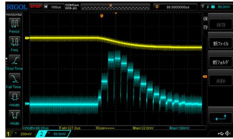
Figure 6: C9 10000 pF, C10 1000 pF detected waveforms.
