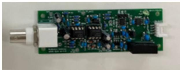
Figure 5: Printed circuit board mounting version(1ch).
