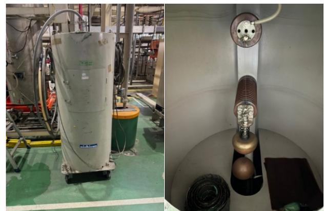
Figure 4: Short-circuit tester (Left: Overall view, Right: Thin copper wire and short-circuit gap inside the short-circuit tester).
