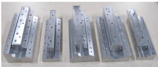
Figure 3: Press molds for outer axis (left), middle axis (second to fourth from left), and inner axis (right).
