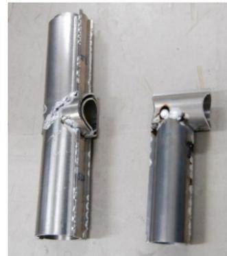
Figure 5: Welded parts of inner axis (right), middle and inner axes (left).
