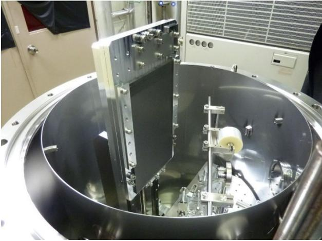
Figure 1: The TIARA laser ion source chamber.
