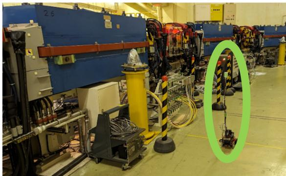
Figure 1: The small-RAT operating inside the ring. An LED light is mounted at the tip of the long rod extending from the top, serving as a visual signal to prevent it from being accidentally stepped on during work.
