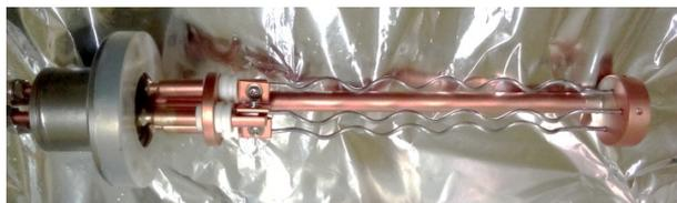
Figure 2: A unused titanium sublimation pump of PF-AR. It has three filaments and a ground, and four terminals outside the vacuum.
