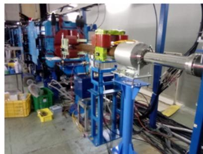
Figure 7: South straight section after the installation of the new DCCT. The cylindrical apparatus near the center of the photograph is the DCCT equipped with an external magnetic shield.
