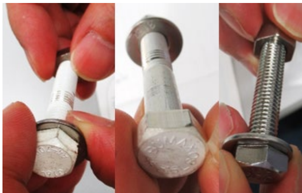
Figure 7: From the left: Teflon-coated silver-plated bolt (SUS316L), Teflon-coated silver-plated bolt (BUMAX), SDC clean bolt (SUS316L) after measurement.
