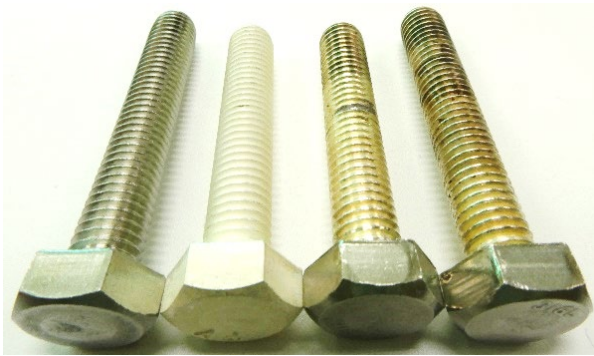
Figure 2: From the left: normal bolt, new, used several times, and used several times and left in the air for a long time Teflon-coated silver-plated bolt (SUS316L).
