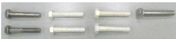
Figure 3: (Upper) From left: normal, silver-plated, Teflon-coated silver-plated, SDC clean bolt (SUS316L). (Bottom) From left: normal, silver-plated, Teflon-coated silver-plated, (BUMAX).
