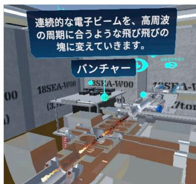
Figure 3. Electrons are accelerated and form bunches. The energies of the electrons are indicated by colors, mapped from black to white.
