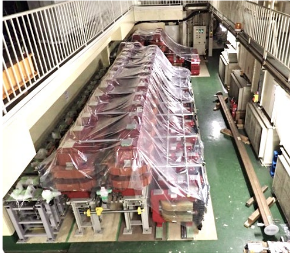
Figure 2: The removed wiggler magnets
