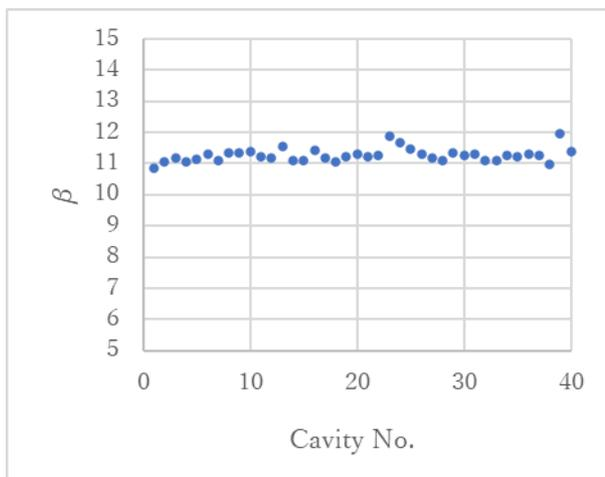
Figure 3: Coupling coefficient  $\beta$  for each cavity.
