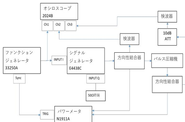
Figure 9: Block diagram of the pulse compression measurements.
