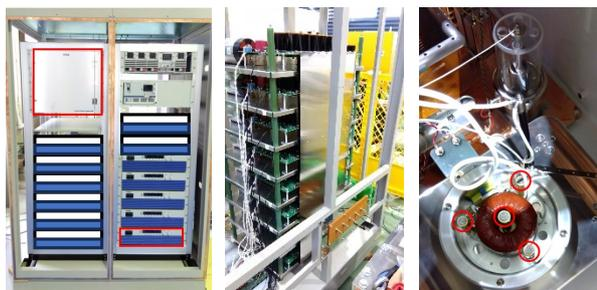
Figure 4: Interior. From left, (a) Charger and control unit. (b) MARX stack. (c) Klystron socket in Oil tank.
