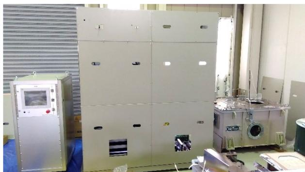
Figure 3: Exterior of modulator. From left, Control rack, High voltage stand(HVS), Oil tank.
