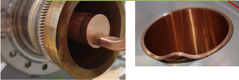
Cu layer on SUS input flange not well attached, RF enter gap and create loop, which further melt and deform. Heat marks on the nearby coupler are visible.
