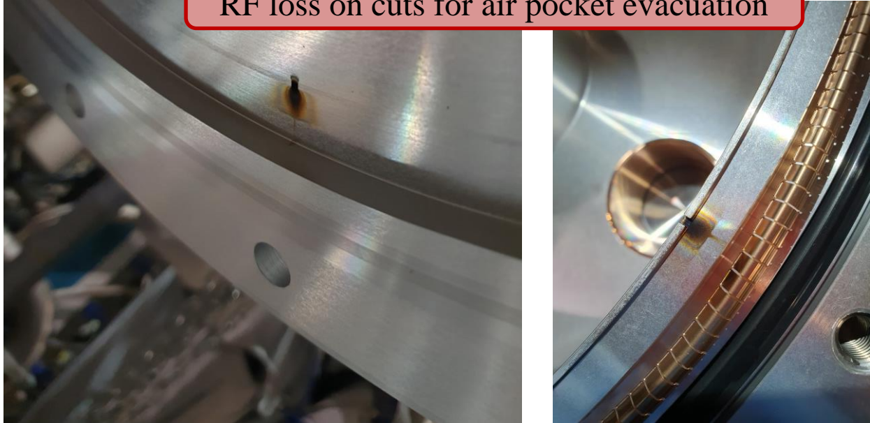
RF loss induced heat in the cuts used for evacuation of air pocket near O-ring.
