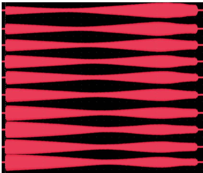
Rev pulse shape for different resonant frequency adjusted with tuner.
