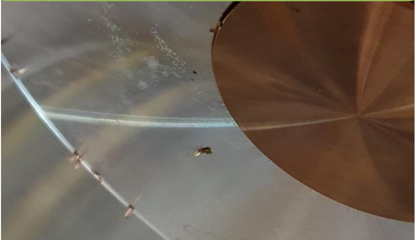
Traces of MP on cavity surface near tuner. Also, visible deformed and melted RF fingers.
