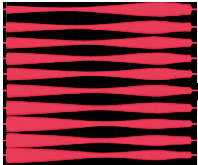
Figure 3: REV pulse shape for FWD = 220 kW, PW = 1 ms, RP = 20 ms; From top to bottom the cavity tuner is linearly swept to change cavity resonant frequency by a total of \sim 30 kHz.
