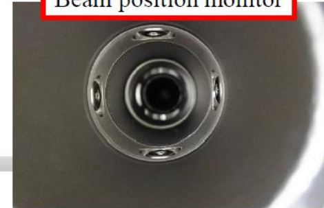
Beam position monitor
