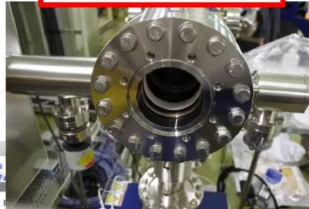
Beam current monitor
