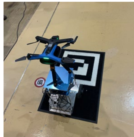
Figure 7: Drone landing base on transport robot.
