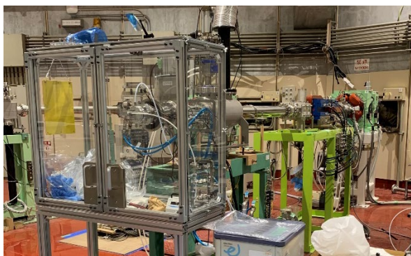
Figure 1: New target system for ^{211}\text{At} production. The blue colored magnets are for beam scanning.
