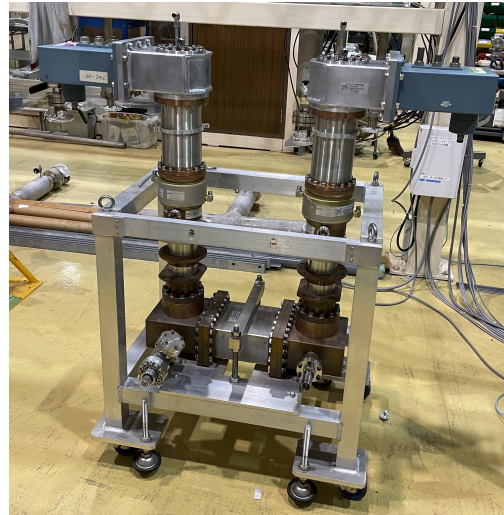
Figure 1: cERL injector prototype coupler test stand.
