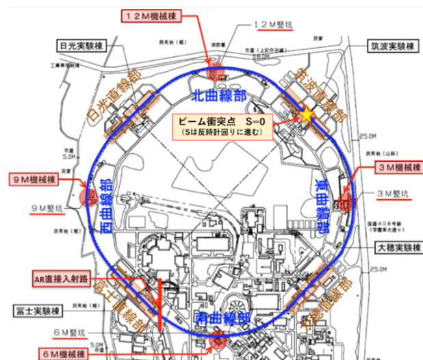
Figure1: SuperKEKB main ring indicated in blue and the construction sites on the ground surface.
