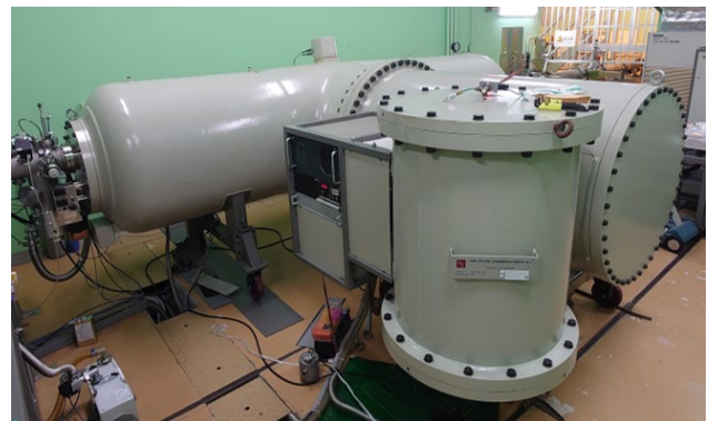
Figure 1: Photograph of Tandetron accelerator.
