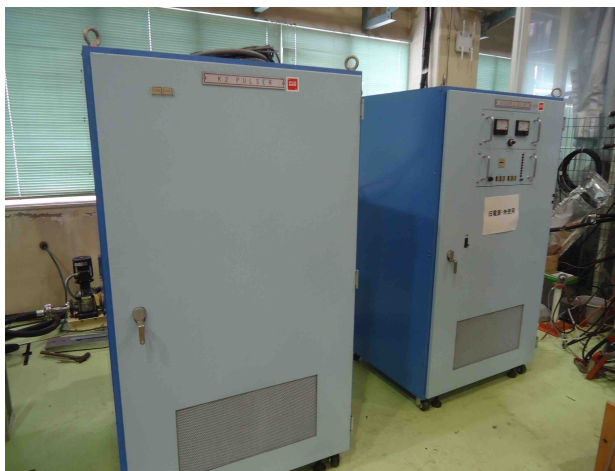
Figure 2: Picture of a kicker test bench which was used as the injection kicker of PF storage ring of KEK.
