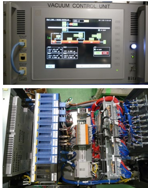
Figure 4: Appearance and interior (LINAC-PLC-VAC).
