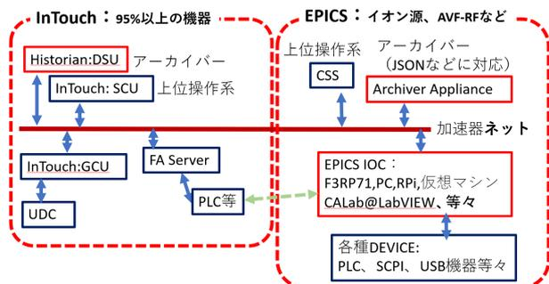
Figure 1: Overview of current control system at RCNP.
