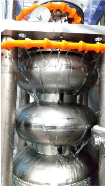
Figure 4: Cavity cooling with pure water.
