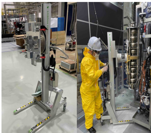
Figure 1: Electric lifter for cavity transport (left) and installation of 9-cell cavity in the EP bed (right).
