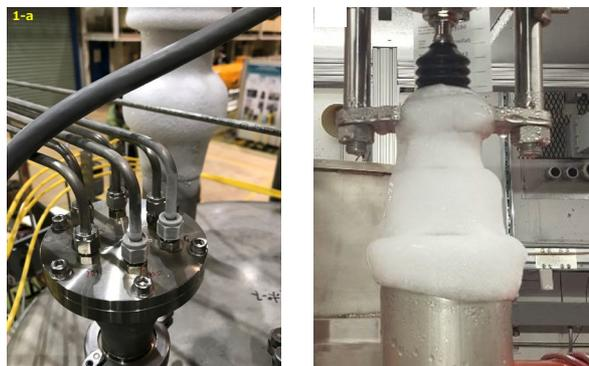
Figure 1: Case samples of thermal oscillation in KEK and FNAL.
