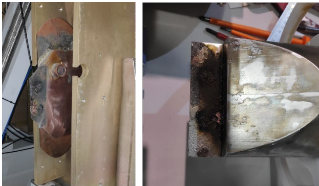
Figure 4: Broken part of the circulator port-1 (2022/Jan).
