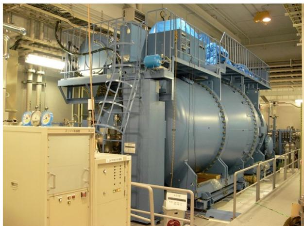
Figure 2: Tandem accelerator.
