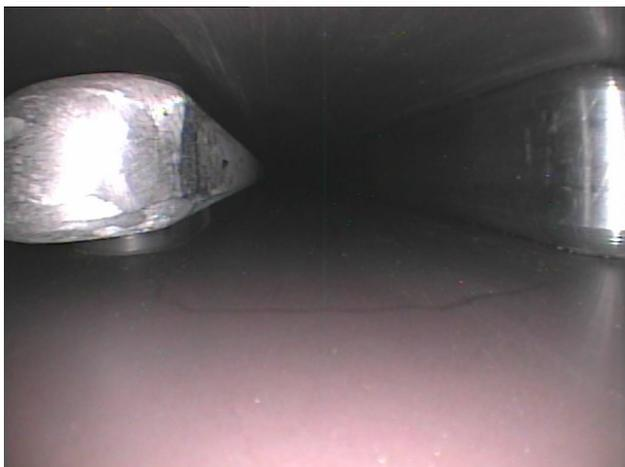
Figure 4: Examples of discharge mark. Upper picture shows the discharge in the insulator and the lower the creep discharge on the surface of the insulator. Both the discharge cases caused burnout of the diode stacks.
