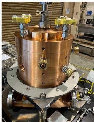
Figure 4: Fabricated SCPC with the frequency tuners.
