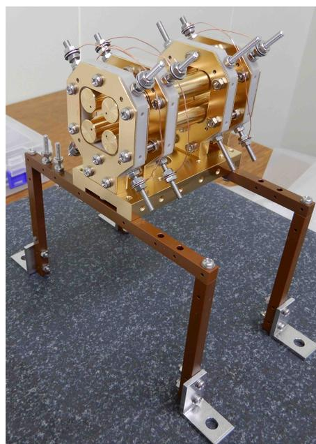
Figure 5: The constructed ion trap.
