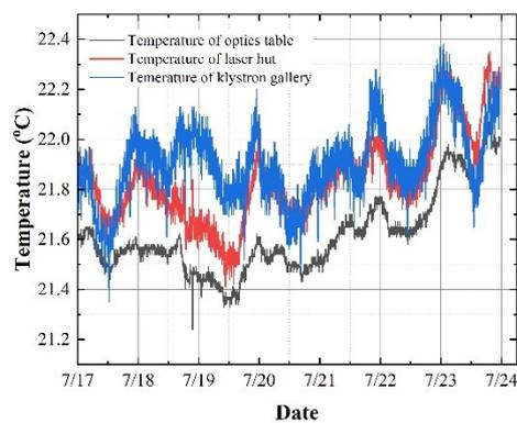
Figure 1: One week temperature history in the laser hut and klystron gallery at Linac.
