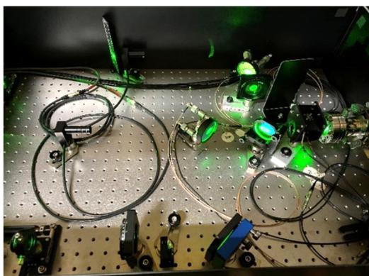
Figure 3: Laser beam position sensor.
