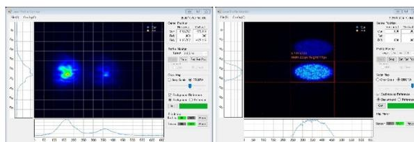
Figure 5: Reshaping for laser beam spatial distribution by the DOE and lens.
