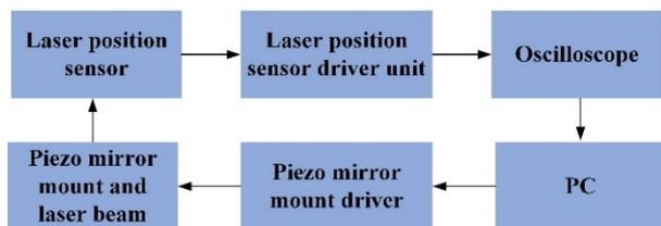
Figure 2: Feedback flow diagram.
