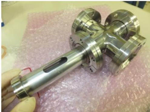
(a) Inner shield of vacuum ports
