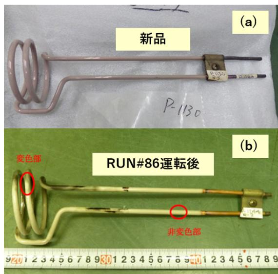
Figure 3: Photos of the RF antenna coils (a) brand new and (b) used in the long-term operation (RUN#86).
