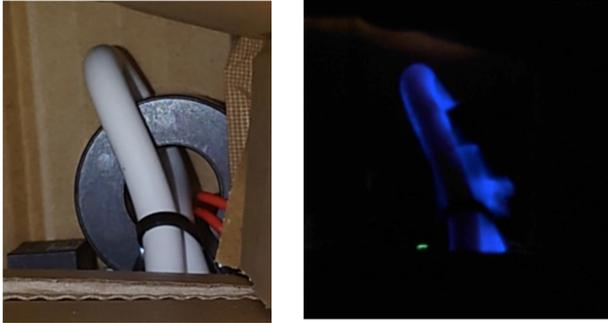
Figure 7: Corona discharge between a high-voltage silicon cable and ferrite core transformer at a voltage of 43 kV, a pulse width of 400 ns and a repetition rate of 50 Hz.
