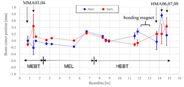
Figure 6: Beam center positions at each quadrupole magnet after the BBA.
