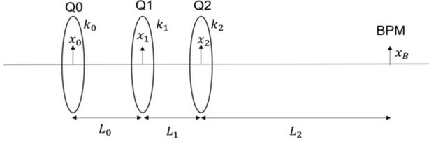
Figure 2: Special configuration of Q0 quad scan for the first one of three quads with a BPM at downstream.
