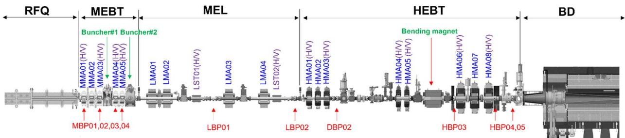
Figure 1: The Phase B+ LIPAc beamline from the exit of RFQ to the entrance of the high-power Beam Dump (BD). Reds: BPMs, blues: quadrupole magnets, purples: steering magnets, greens: bunchers and bending magnet.
