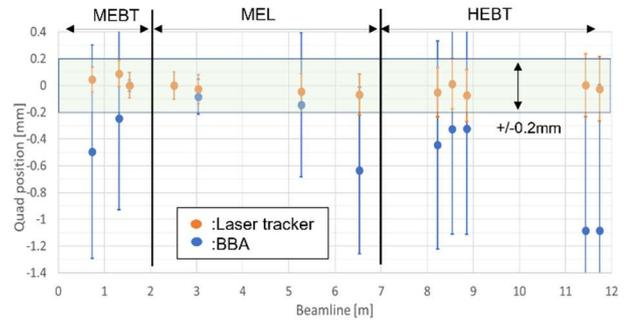
Figure 7: Comparisons of quad positions measured with a 5 MeV beam and the laser tracker system. The left and right plots show the horizontal and the vertical planes. Note that the vertical scales are different in the two plots. Blue and orange colors stand for the results measured by the BBA method and laser tracker system, respectively.
