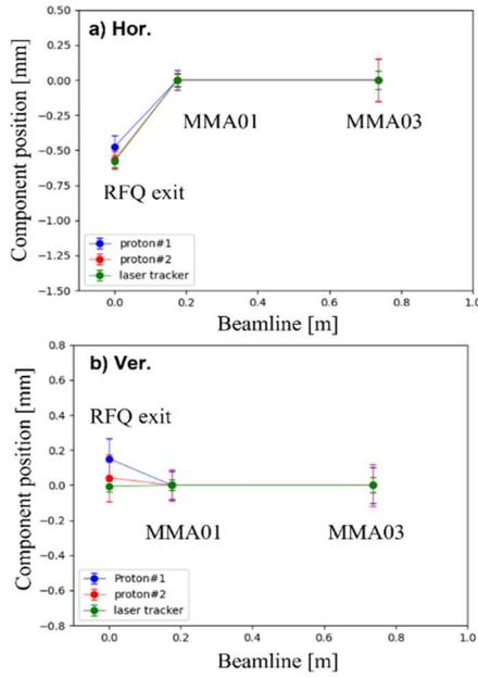
Figure 5: The positions of the RFQ exit, MMA01, and MMA03. a) and b) are the horizontal and vertical positions, respectively. Zero positions in the vertical axes is a line passing through the magnetic centers of MMA01 and MMA03.
