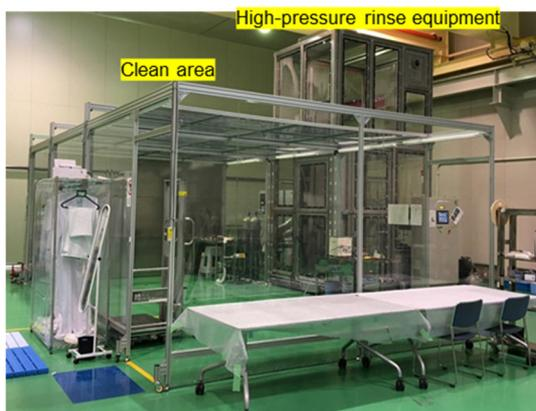
Figure 2: High-pressure rinse facility.
