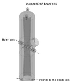
Figure 8: Change the rinsing port layout.
