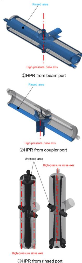
Figure 9: Study results of high-pressure rinsed area.
