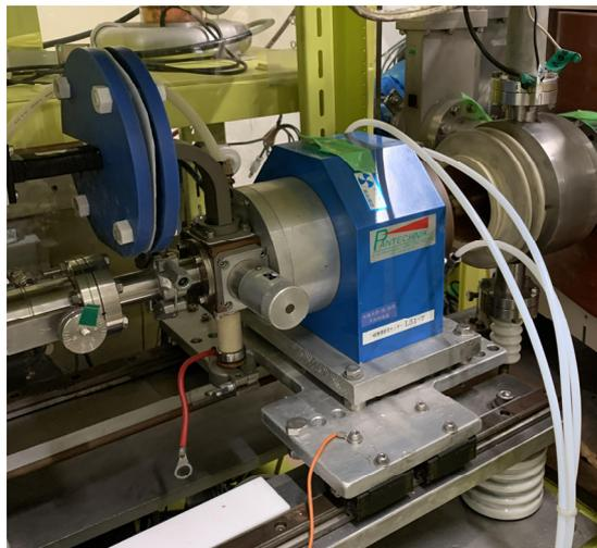
Figure 2: The 10GHz permanent magnet ECR NANOGAN (PANTECHNIK): It has two extraction electrodes. It is possible to apply 15 kV between these electrodes, and it is also possible to apply 35 kV between first extraction electrode and plasma electrode.
