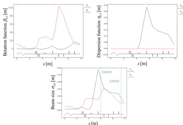
Figure 9: Betatron and dispersion functions (upper) and beam sizes (lower) along the dump line by simulation.
