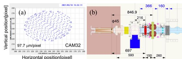
Figure 6: (a) Beam position movement by the rastering magnet at CAM32 and (b) layout near the rastering magnet and the beam dump.
