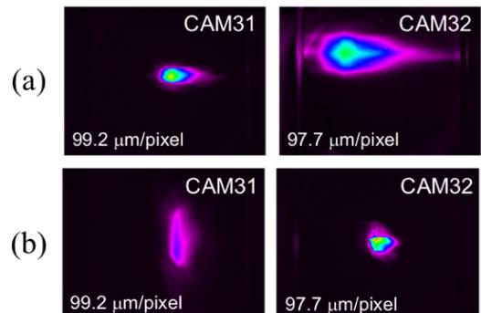
Figure 5: Beam profiles at CAM31 and CAM32 for the 5-MeV beam. (a) QM1-5 were turned off and the beam orbit was tuned by the dump chicane so as to be the position center at CAM31. (b) QM1-5 and their steering coils were excited to tune the beam sizes and positions.
