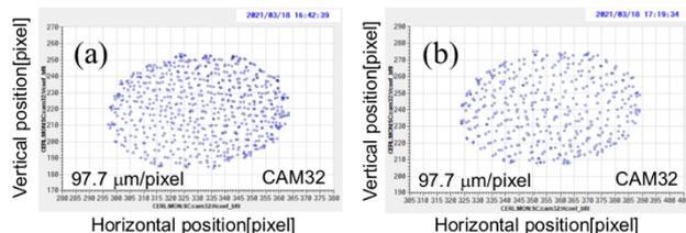
Figure 8: Beam position movement by the rastering magnet at CAM32 with (a) on-crest and (b) off-crest deceleration by the ML2 cavity.
