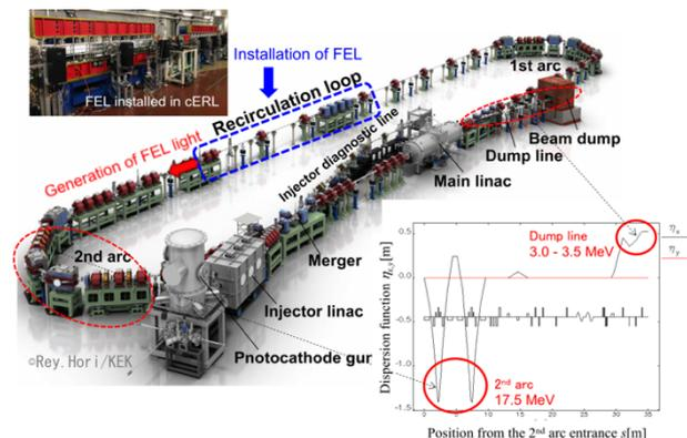
Figure 1: Illustration of the cERL including two dispersive regions, the 2<sup>nd</sup> arc and dump line, downstream of the IR-FEL with the dispersion functions.
