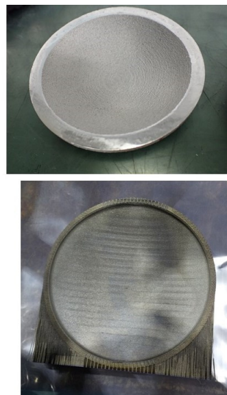
Figure 4: Pictures of the sphere window with a diameter of 60 mm and with a thickness of 0.2 mm (UP) and the window with a diameter of 166 mm and with a thickness of 0.6 mm (DOWN).
