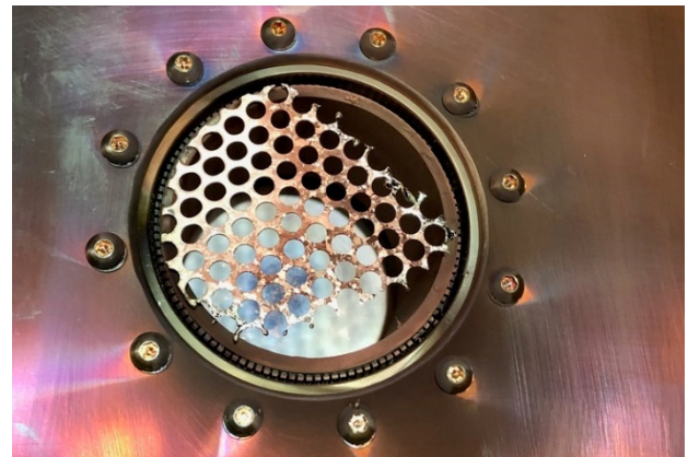
Figure 3: Damaged RF shield.
