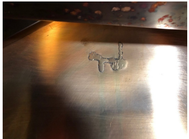
Figure 7: Resonator for RRC repaired in June 2020.
