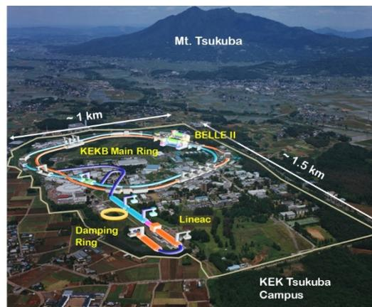
Figure 1: Schematic layout of SuperKEKB at Tsukuba campus.
