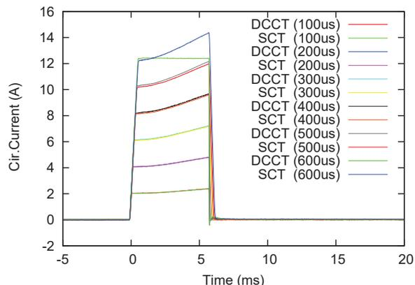
Figure 6: Circulating current of DCCT and SCT.
