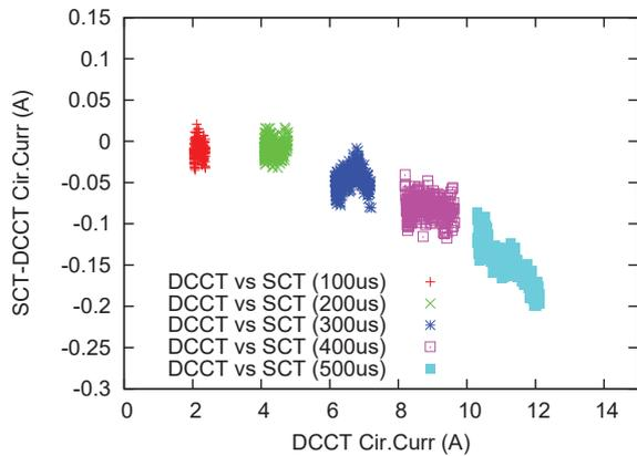
Figure 8: Circulating current correlation between DCCT and SCT.
