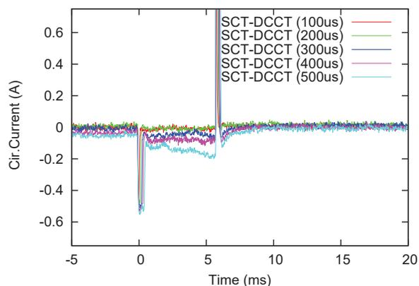
Figure 7: Circulating current difference between DCCT and SCT.
