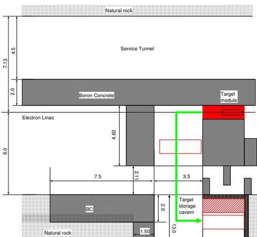
Figure 5: Horizontal view of the upstream part of the target section.
