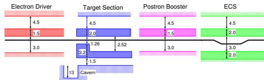
Figure 2: Horizontal layout of each section; From the left to right, Electron driver, the target and capture section, positron booster, and ECS. For all sections, the upper area is the service tunnel where the power source and other hardware are placed in. The lower area is the accelerator tunnel where the accelerator is placed. The exception is the target and capture; The middle is the accelerator tunnel and the lower is the corridor. There is a cavern where the used target module is stored.
